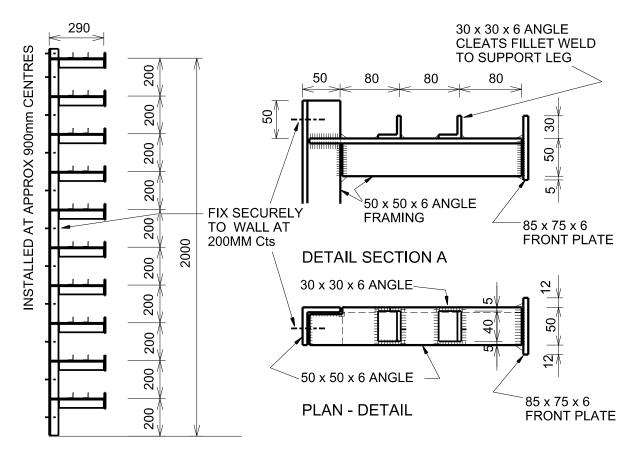
**ELEVATION - OPEN RACKS FOR METAL LENGTHS**
