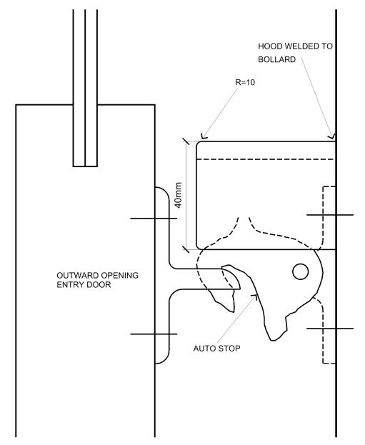
DOOR STOP AND HOLDER LOCATED AT BOTTOM RAIL
